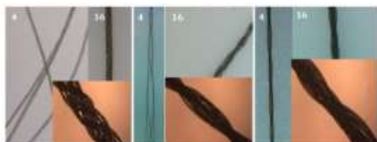
Figure 2. Microscopes images of braid patterns after hydrogel coatings from left to right: 1x1 and 2x2 biaxial; 1x1 triaxial patterns.
