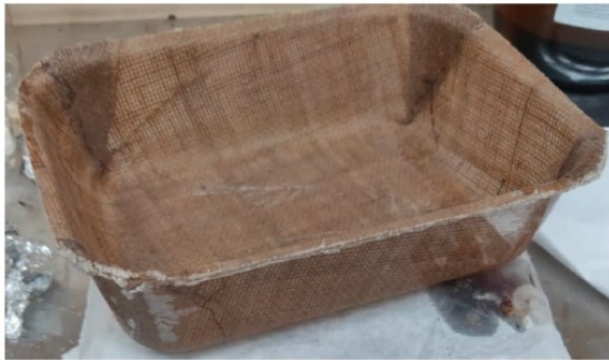
Figure 3. natural fibre reinforced polymer composite tray from vacuum bagging
