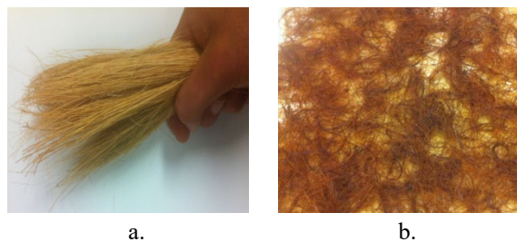
Figure 1. Date palm fibers preparation, a. PDPFiber after extraction, b. PDPFiber after treatment
