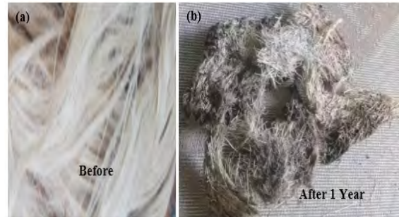
Figure 4. Biodegradability test of textile materials reinforced composite in soil for one year a) Neat enset fiber reinforced green composite b) Green composite material after one year left in soil.
