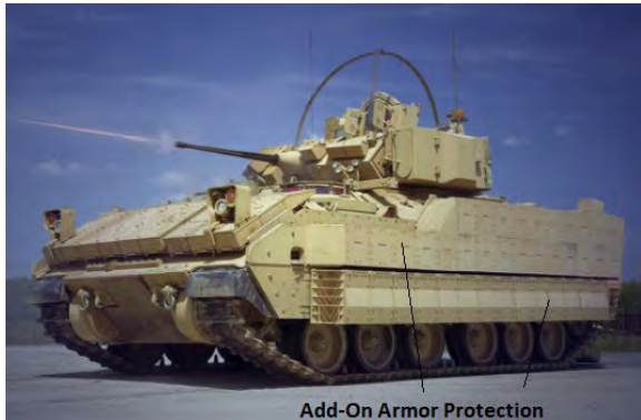
Figure 7. An armored vehicle under add-on armor protection
