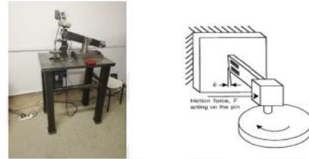
Figure 3. a-Abrasion Test Device, b-Schematic Representation [8]
