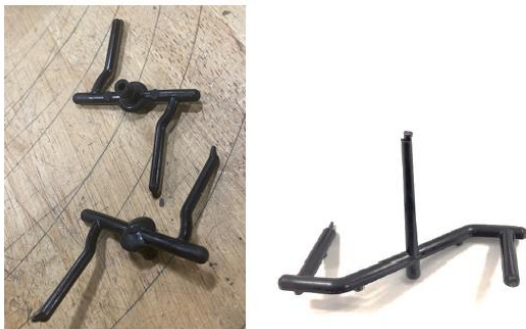
Figure 2. Injection sprue and runner (industrial waste)
