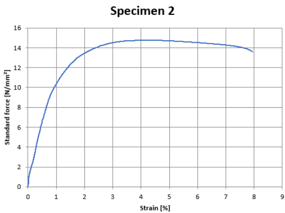
Figure 4b. Tensile test result of specimen 2
