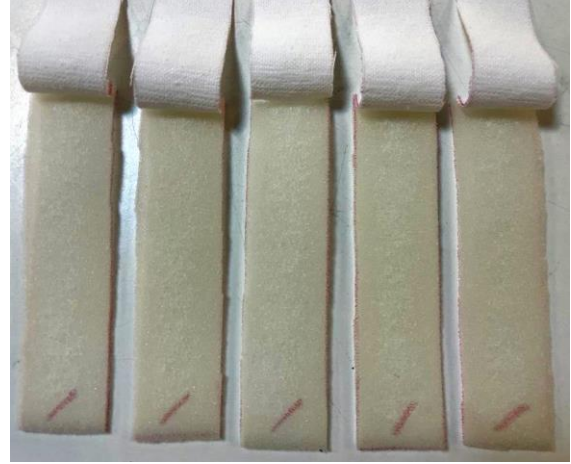
Figure 2. Surface of the foams after bond strength test
