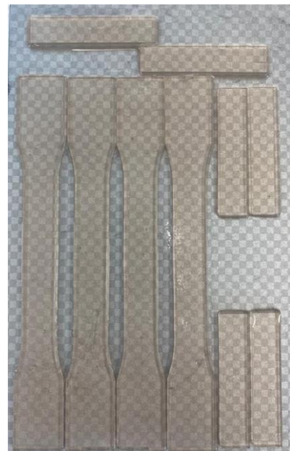
Figure 2. Layout of nanocomposite specimens on the printing bed.
